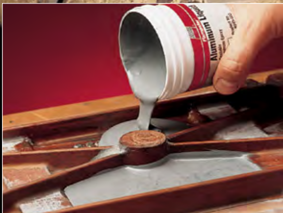
Pouring moulds with Fixmaster® Aluminium Liquid
