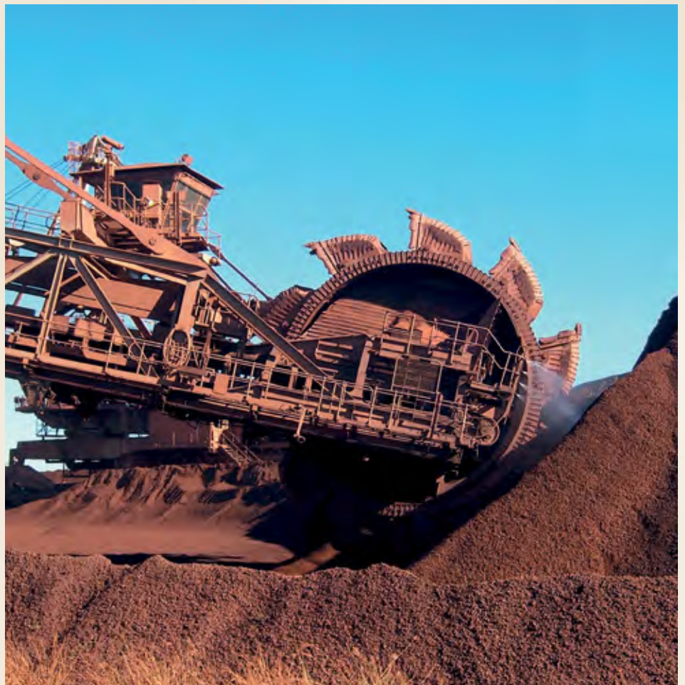
Reclaimer buckets are subject to excessive and constant wear
