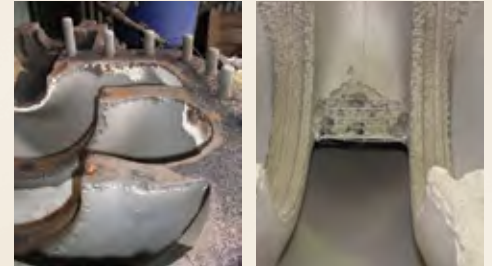
Pitting and erosion was clearly evident
