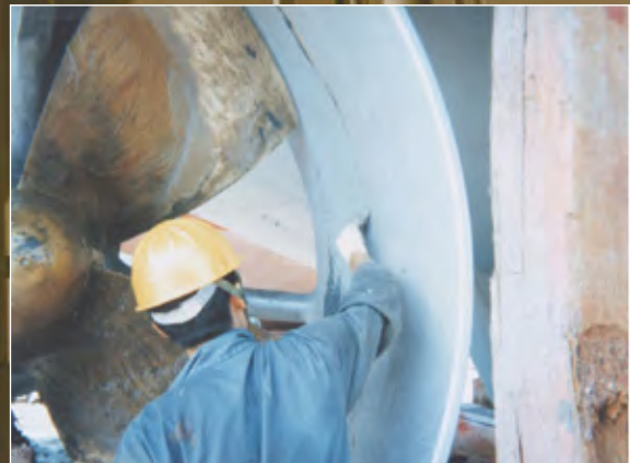
Applying Nordbak® Brushable Ceramic to an impeller
