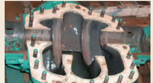
Pitting and erosion was clearly evident
